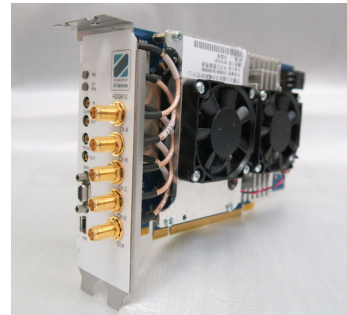
Figure 6: Outward of ADQ412 with PCIe form factor.
