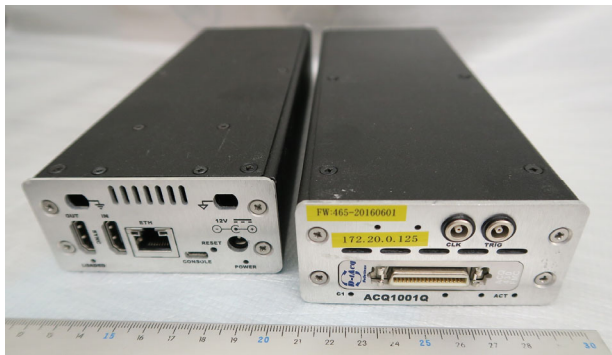
Figure 4: Outward of ACQ1001 with FMC module.
