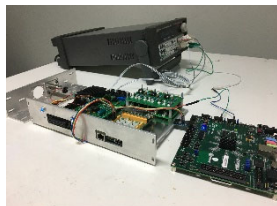
Figure 3: Test setup for PWM drive PCB with Zedboard controller and DC power supply.
