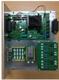
Figure 2: Custom PWM drive PCB installed in a standard equipment box.
